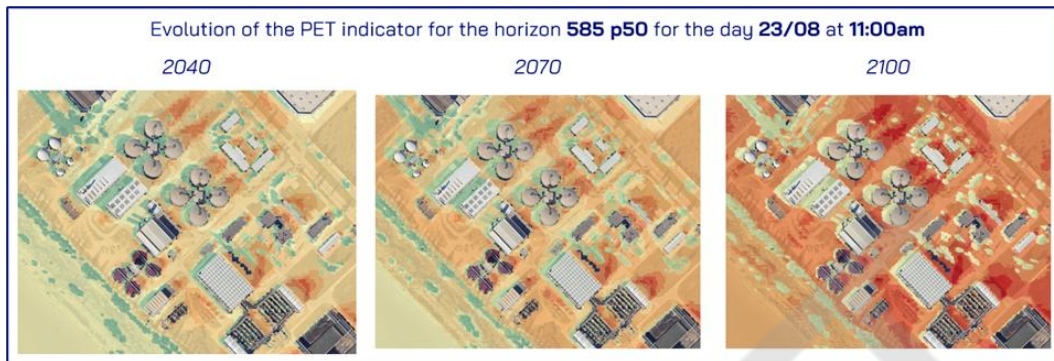
Figure 24. Evolution of the PET indicator for the horizon 5-8.5 p50 for the day 23/08 at 11:00 am.
