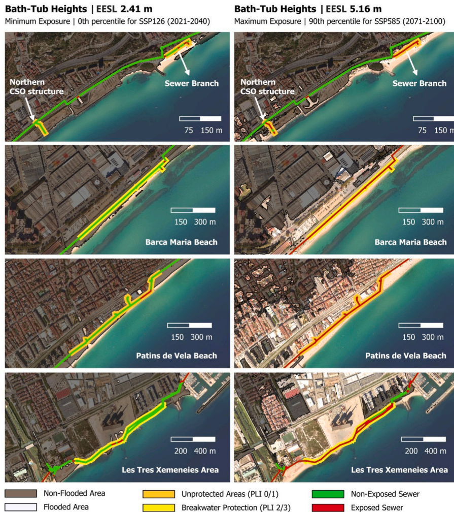
Fig. 9. Most favourable and critical situations of projected coastal flooding events (EESL water height) for 2015-2100 for unprotected areas (PLI 0/1) and rock revetment protection (PL 2/3) of the Llevant Main Sewer. The sections shown correspond to those identified as potentially exposed and presented in Fig. 7.
